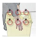
A sound ensures that the clip has been correctly inserted and the clip can be seen in the edge of the lid
