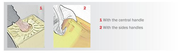
WARNING: With lid DUO N, use the central handle only with screw lid in permanent closure. Do not use the central handle of the screw lid in temporary closure
