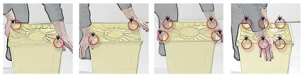
A sound ensures that the clip has been correctly inserted and the clip can be seen in the edge of the lid
