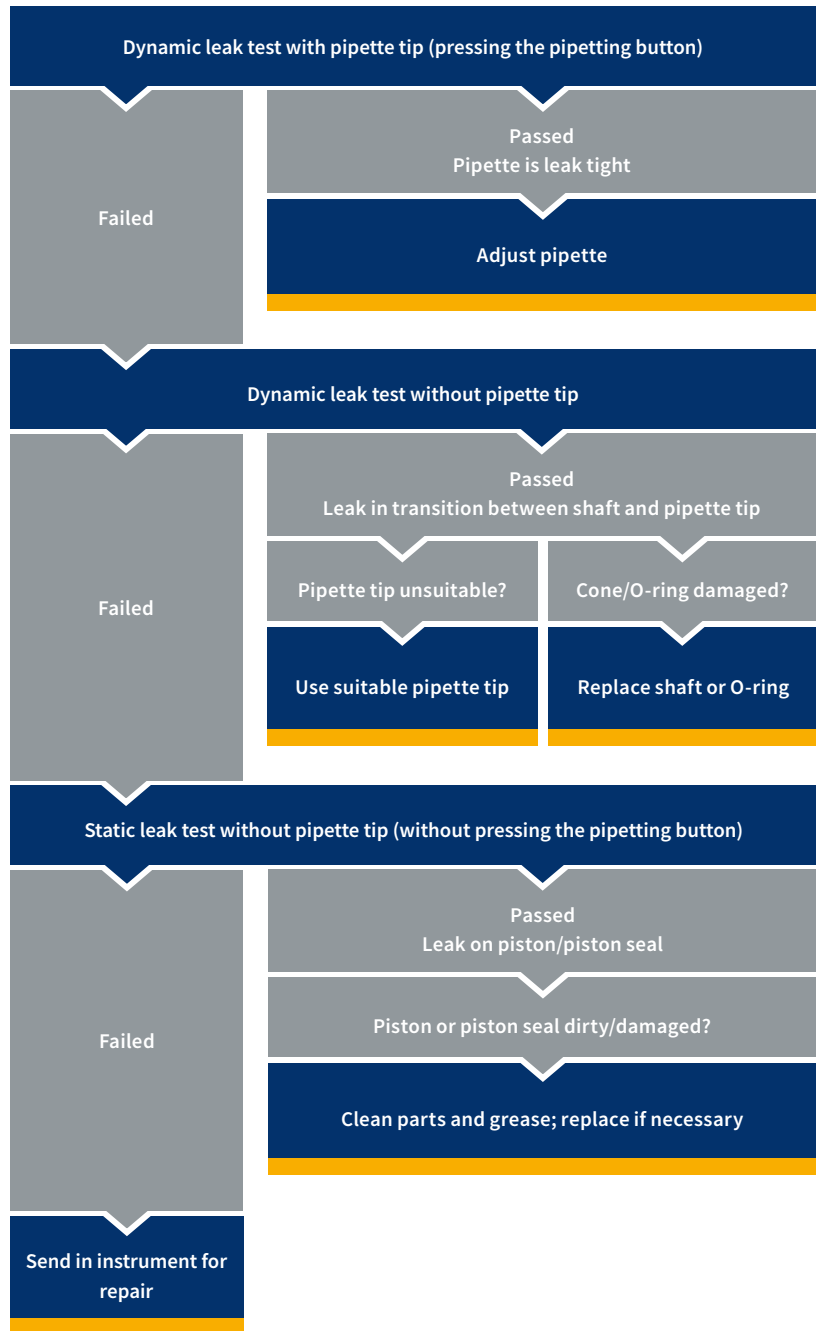
Figure 2 Determining a pipette cause for the leak with the BRAND PLT unit
