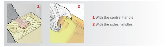
WARNING: With lid DUO N, use the central handle only with screw lid in permanent closure. Do not use the central handle of the screw lid in temporary closure
